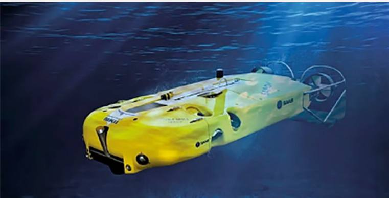
This unmanned underwater vehicle is a Double Eagle from the Swedish defence company Saab and is used to detect and neutralise naval mines.
